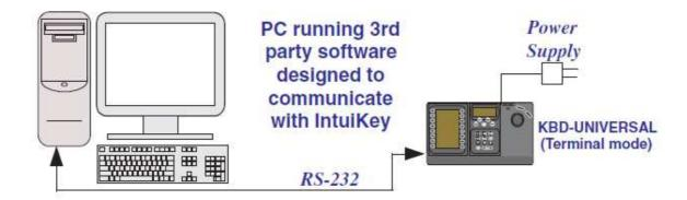
This connection requires a standard Null modem RS-232 link. If desired, the Bosch Security Systems cable S1385 can be used. Connect one end of the RS-232 interface cable to the 9-pin RS-232 Serial Port located on the far right side of the rear of the KBD-Universal keyboard. Connect the other end of the RS-232 interface cable to a COM port on the PC.
