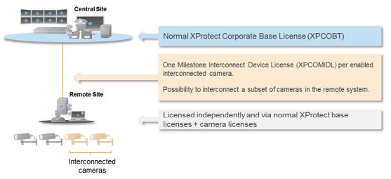
As indicated in the figure above, it is possible to interconnect a subset of cameras in an interconnected system. Please note that an interconnected remote system without any enabled cameras will require one Milestone Interconnect Device License.
